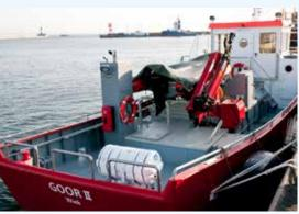
**FS "GOOR II"s** hull is made of steel with 9 up to 11 mm thickness. The cooling of the engine is trough pockets in the hull. This is very safety and environmentally friendly. The GOOR II is very manoeuvrable (bowthruster) and with a specialized anchor-system (up to 3 anchors) equipped.
